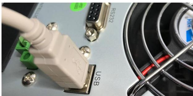
The USB port provides full serial communications to an attached computer. Being HID compliant the unit will "talk" to the operating system directly (effectively making a desktop like a laptop in terms of power operation). Alternatively, shutdown software can be downloaded and installed.
