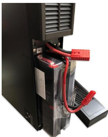
The UPS internal batteries as well as the cabinet batteries are contained within self contained trays and are fully hot-swappable.
