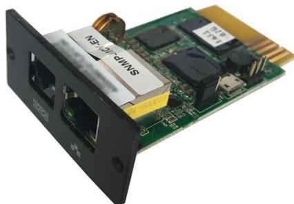
The rear panel includes an "intelligent slot" for the addition of either an SNMP or an AS400 relay card. SNMP allows monitoring of the UPS over a network connection. The advanced card also contains an event log. The relay card allows connection to AS400 servers or any other remote alarm or Building Management Systems.
