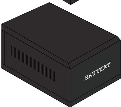
3. Fit the right and left side panels. They fit into the grooves with the front and rear panels. Finally fit the lid.
