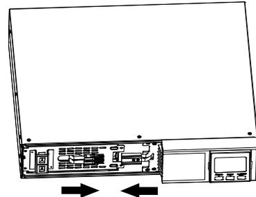
Re-connect the battery wires.
