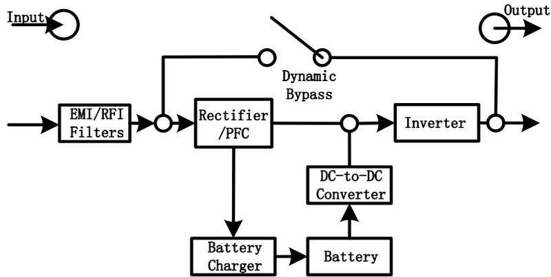
The UPS is composed of mains input, EMI/RFI filters, rectifier/PFC, inverter, battery charger, DC-to-DC converter, battery, dynamic bypass and UPS output.
