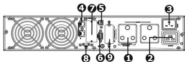
1. Programmable outlets: connect to non-critical loads.
